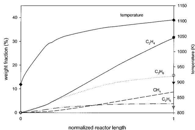
**Figure 5.** Comparisons between simulation results and operating data. Lines denote simulation data, and symbols denote operating data.
