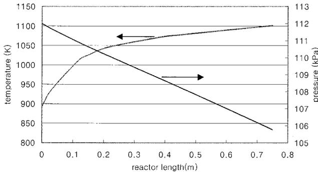
**Figure 3.** Comparison of temperature and pressure between full and reduced reaction models.
