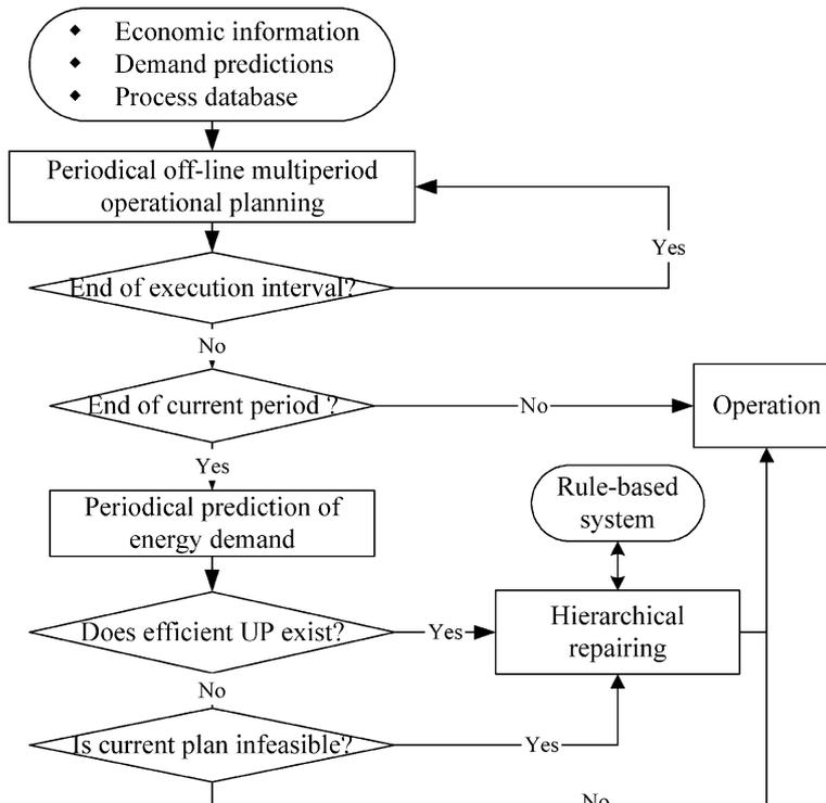
Fig. 4. The integration methodology of the periodical replanning and the hierarchical repairing for the optimal operation.
