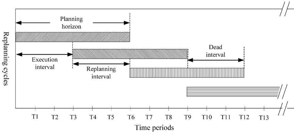
Fig. 1. Periodical replanning cycles in continuous plant.
