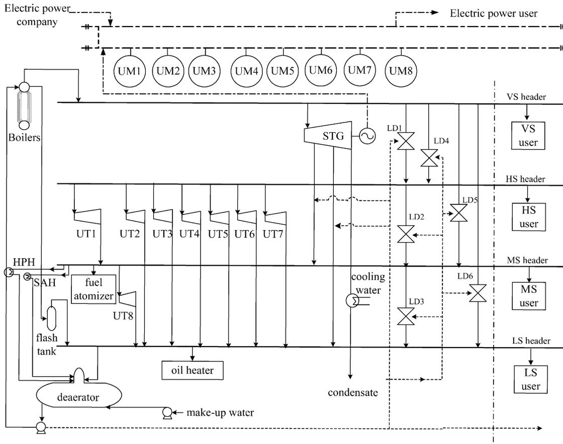
Fig. 5. The schematic diagram to show the process flow of an industrial utility plant.
