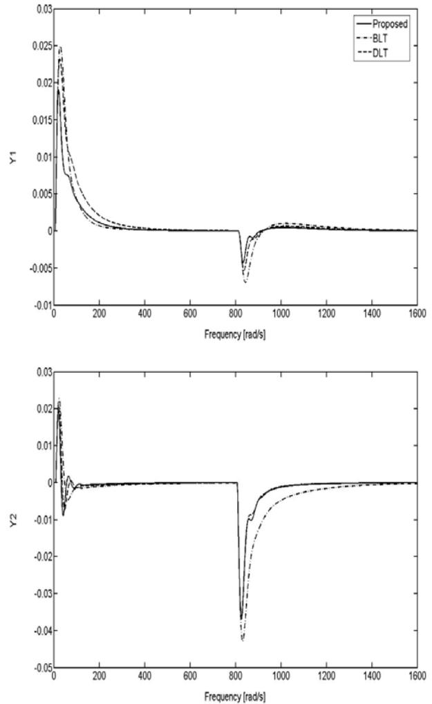
Fig.4 Closed-loop response to sequential step changes in disturbance for WW column
