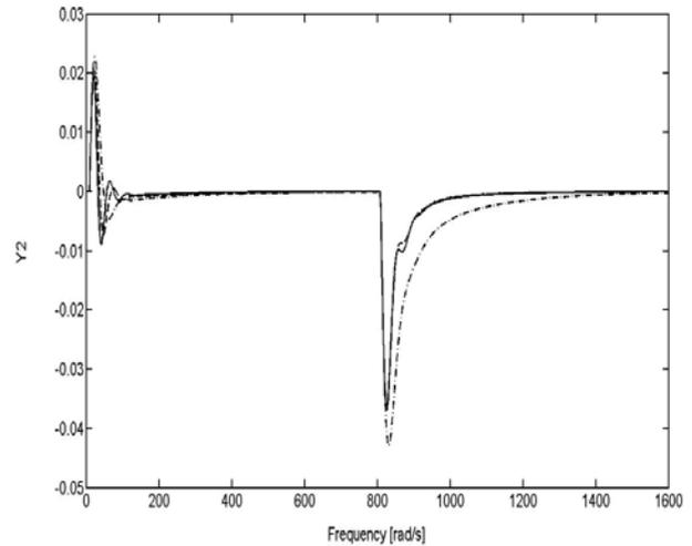
Fig.4 Closed-loop response to sequential step changes in disturbance for WW column
