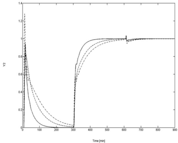
Fig.5 Closed-loop response to sequential step changes in set-point for OR column
