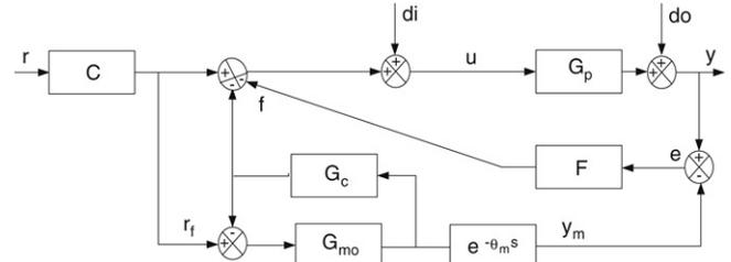
Fig. 1. Two-degree-of-freedom control structure by Liu et al. [8].
