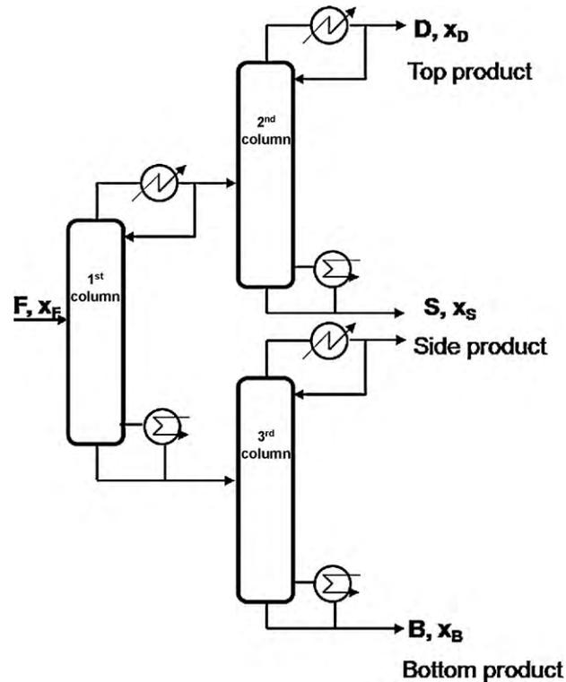
Fig. 7. Schematic diagram of a three-column distillation system for initial design of DWC structure.
