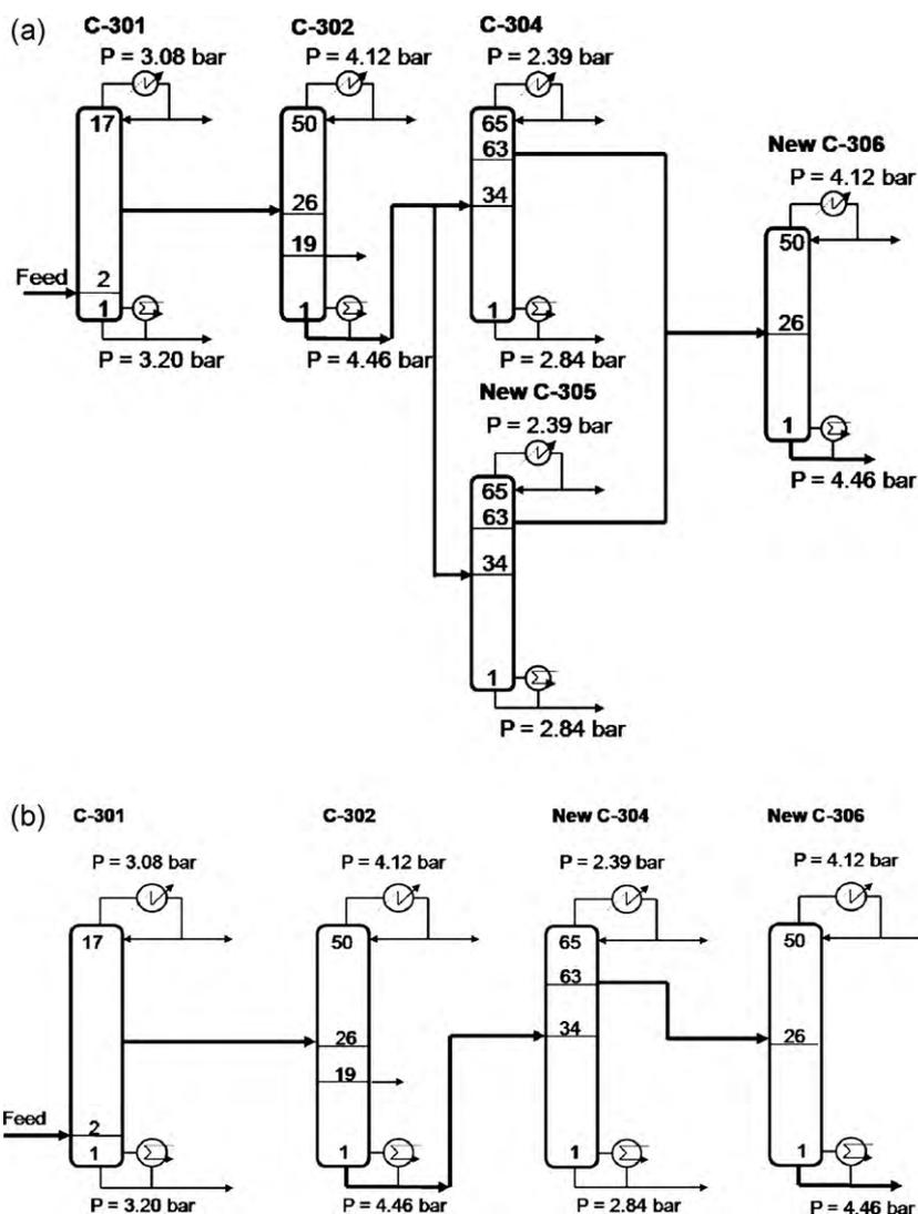
Fig. 4. Simplified flow sheet illustrating the separation train showing: (a) five conventional columns, including one new column added in parallel with C-304 and another added in series and (b) four conventional columns, including a new C-304 and one new column added in series.
