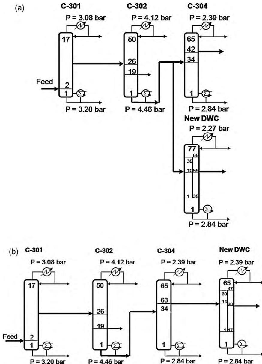
**Fig. 9.** Simplified flow sheet illustrating the separation train, showing four columns, including the additional DWC: (a) parallel with C-304 and (b) in the series.
