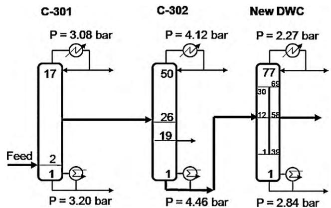
Fig. 6. Simplified flow sheet illustrating the separation train, including a two conventional column distillation and one DWC system.
