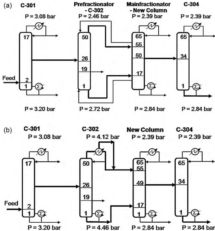
Fig. 5. Simplified flow sheet illustrating the separation train, including: (a) the Petlyuk arrangement and (b) the prefractionator arrangement by adding a new column.
