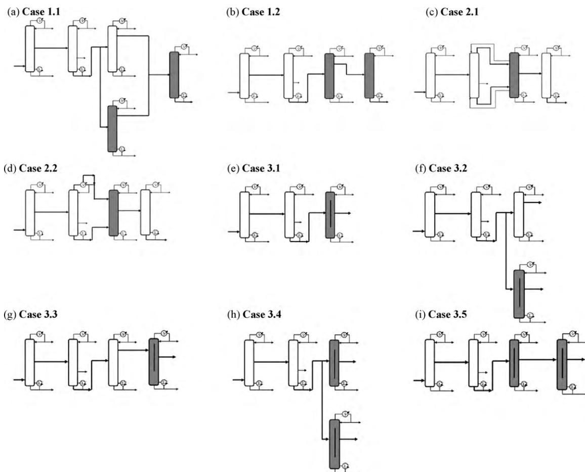
Fig. 3. The nine separation trains explored for column debottlenecking. All the gray columns are new columns or existing columns retrofitted to a DWC.
