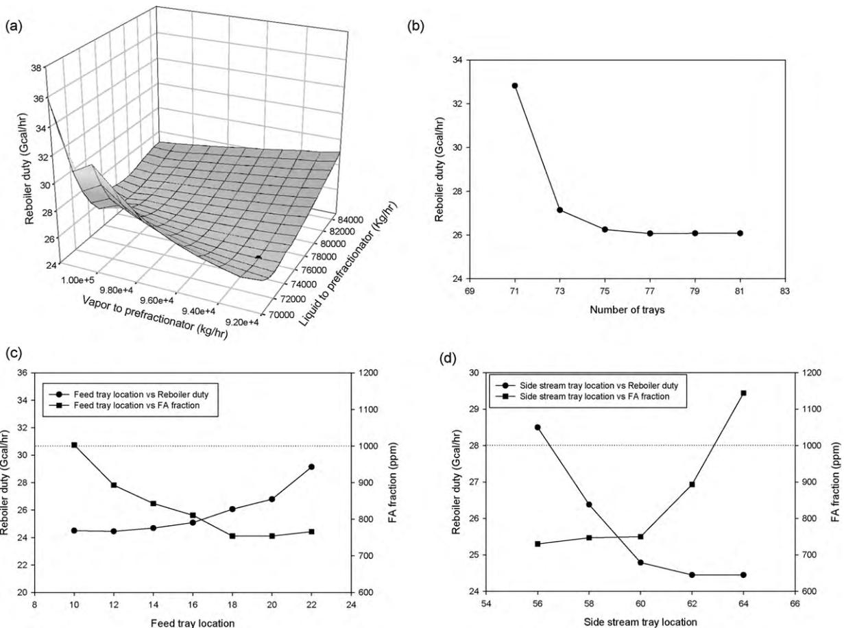
Fig. 8. Effects of: (a) liquid and vapor flow into the prefractionator section; (b) the number of trays of the main fractionator; (c) the feed tray location; and (d) the side tray location on the reboiler duty of the DWC.
