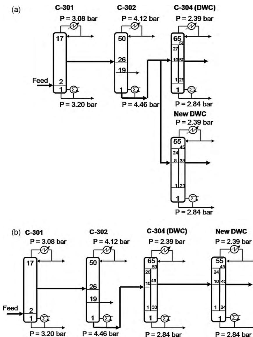
Fig. 10. Simplified flow sheet illustrating the separation train showing: (a) two conventional distillation columns and two DWC systems, including one from retrofitting C-304 and one new DWC, parallel with the C-304 and (b) two conventional distillation columns and two DWC systems, including one from retrofitting C-304 and one new DWC in series.
