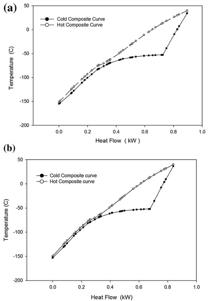
Fig. 4. Composite curves for (a) base case and (b) PSP optimized case.
