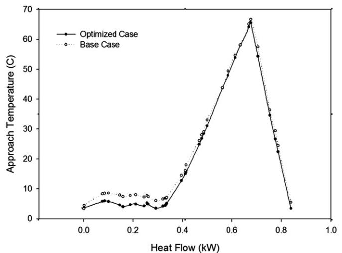
Fig. 5. Approach temperature variation within a heat exchanger.
