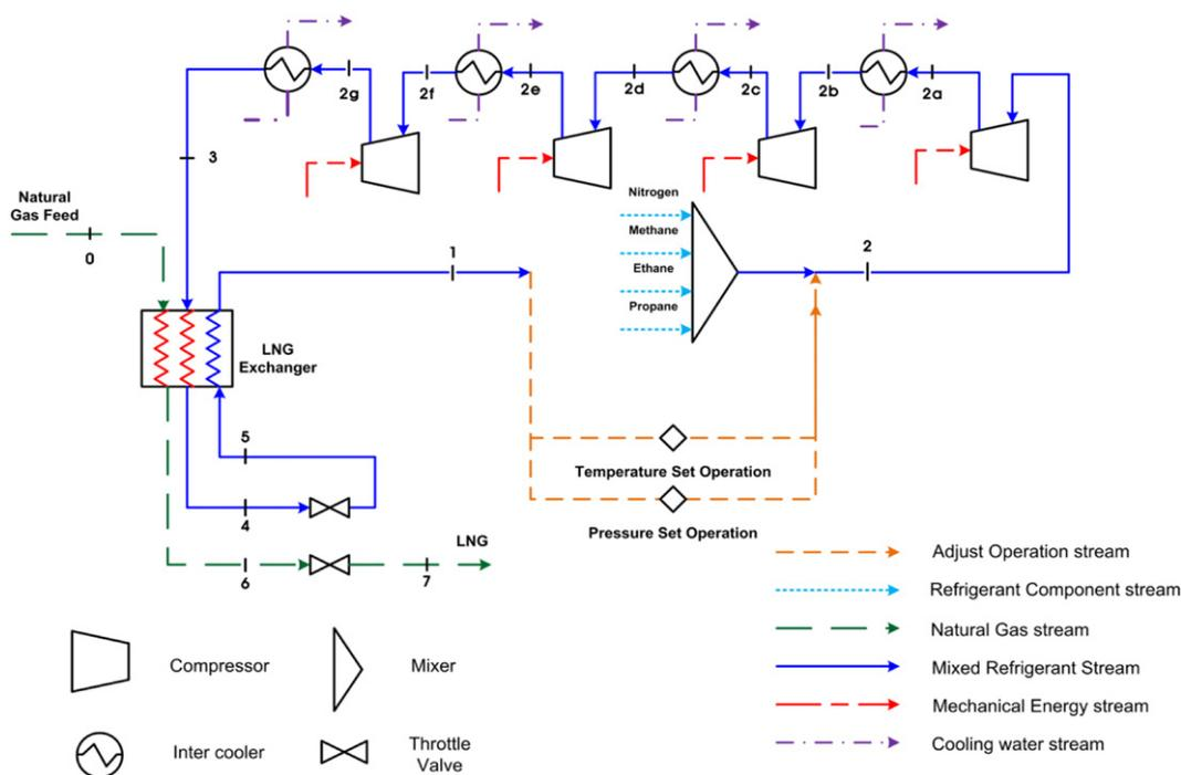
Fig. 2. Schematic diagram of SMR process.
