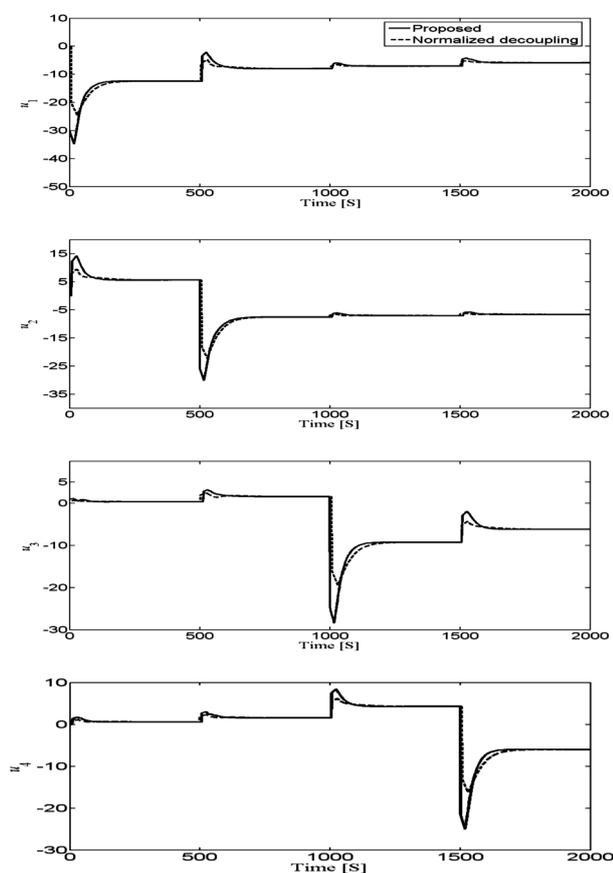
Fig. 9 Controller output responses to the sequential unit step changes in the set-point for the HVAC system
