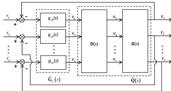
Fig. 1 Block diagram of a decoupling control system
