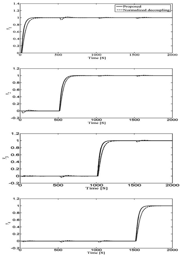
Fig. 8 Closed-loop responses to sequential step changes in the set-points for the HVAC system
