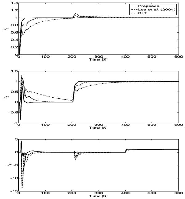
Fig. 6 Closed-loop responses to sequential step changes in the set-points for the OR column
