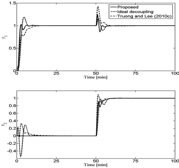
Fig. 5 Closed-loop responses to sequential step changes in the set-points for the VL column
