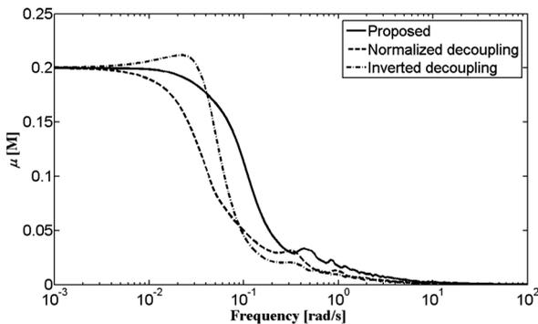
Fig. 7 SSV plots for robust stability in HVAC system
