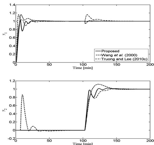
Fig. 4 Closed-loop responses to sequential step changes in the set-points for the WB column
