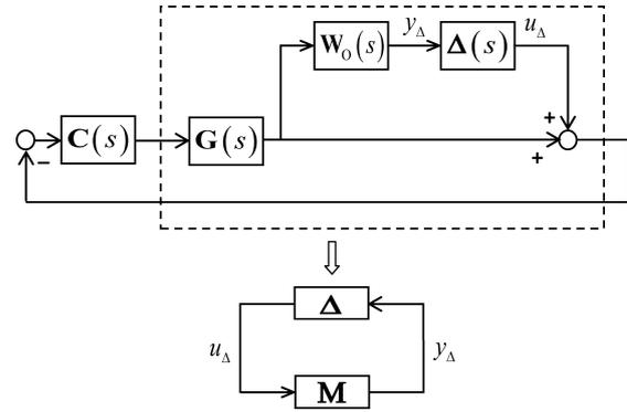
**Fig. 2** Control system with multiplicative output uncertainty and its  $\mathbf{M}-\Delta$  control structure for robustness analysis
