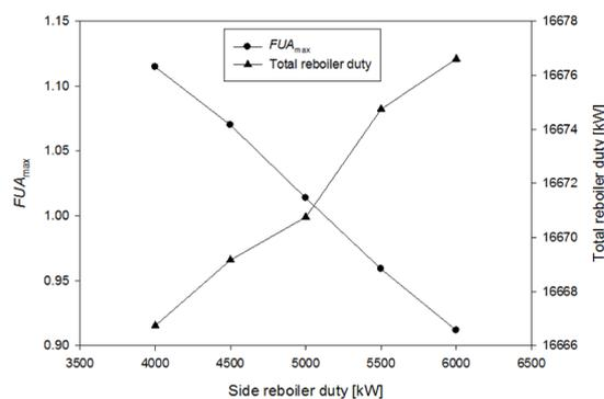
Fig. 9 Influence of side reboiler duty on the total reboiler duty,  $FUA_{max}$
