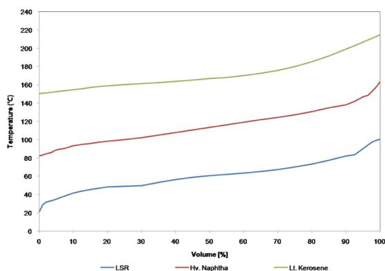
Fig. 2 Naphtha splitting column—ASTM D86 curves of the distillates
