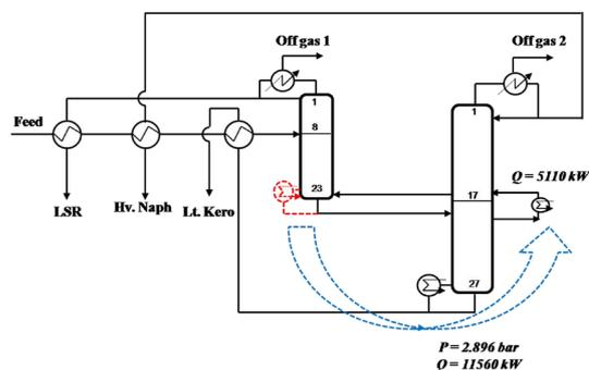
Fig. 8 Simplified flow sheet illustrating the retrofitted TCDS with side reboiler
