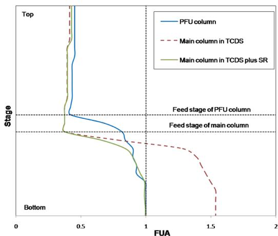
Fig. 7 FUA profiles of existing PFU and main column in TCDS
