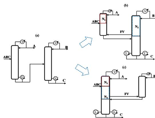
Fig. 3 Schematic diagram of the (a) Existing direct sequence; (b) Thermally coupled direct sequence with side rectifier and (c) Equivalent side rectifier arrangement
