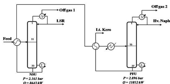
Fig. 1 Schematic diagram of the naphtha splitter process
