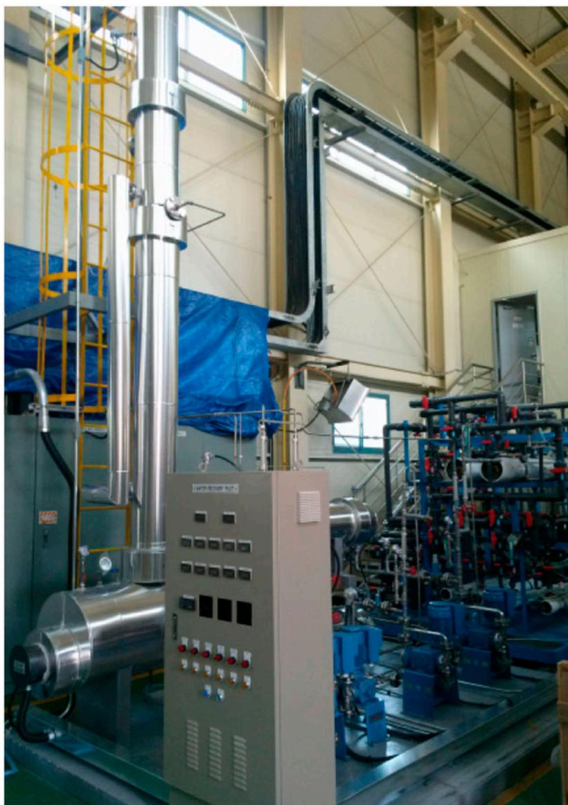
Fig. 2. Forward osmosis desalination pilot system at KIMM.
