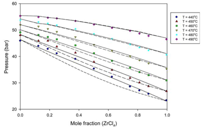
Fig. 4. P-xy diagram at different temperatures for the  $ZrCl_4/HfCl_4$  system: the symbols denote experimental bubble points, and the solid and dashes lines are the bubble point and dew point curves correlated by the PR-EOS, respectively.
