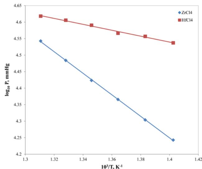
**Fig. 3. Vapor pressure of  $ZrCl_4$  and  $HfCl_4$ .**
