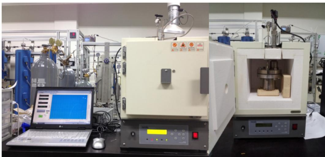
Fig. 1. Experimental apparatus for determining the bubble point pressure of a binary mixture.
