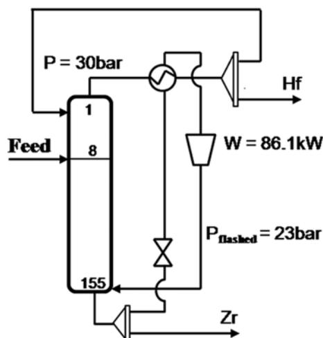
Fig. 7. A flow sheet diagram illustrating the partial bottom flashing heat pump.
