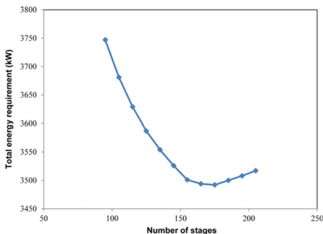
Fig. 6. Sensitivity analysis between the number of stages and the total energy requirement for the high pressure distillation column.
