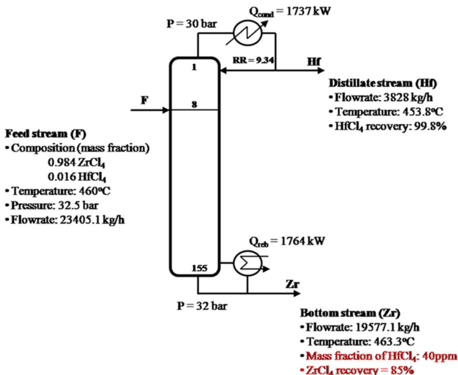
Fig. 5. A flow sheet diagram illustrating the high pressure distillation column.
