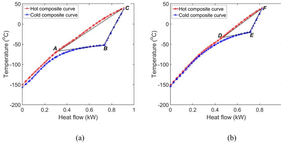
Fig. 1. Composite curves of a) conventional mixed refrigerant; b) with the addition of n-butane.
