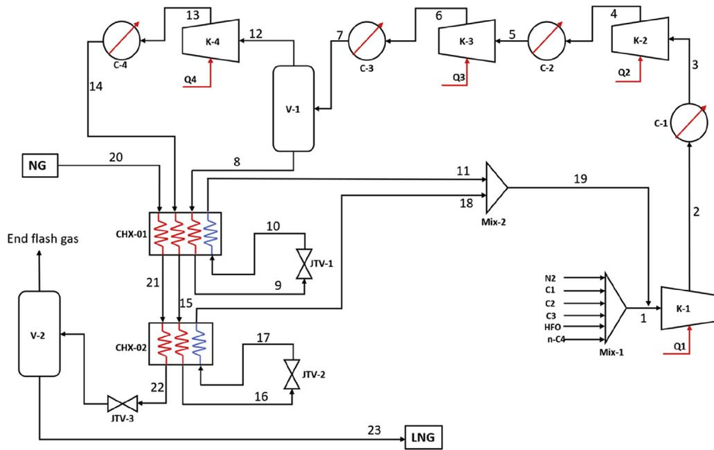
Fig. 2. Process flow diagram of HFO-MR natural gas liquefaction process.
