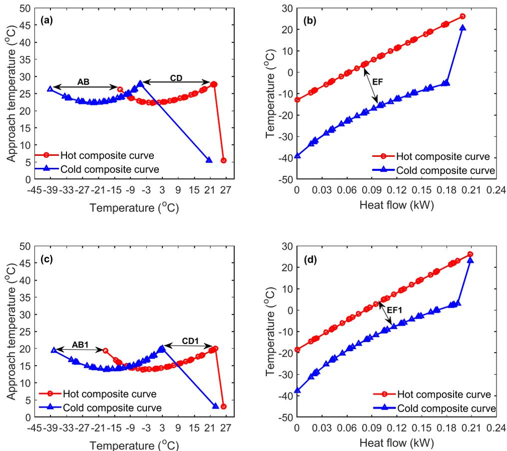
**Fig. 5.** TDCC and THCC in the precooling exchanger (CHX-01) of the HFO-MR LNG process, without optimization (a and b) and with optimization (c and d), respectively.
