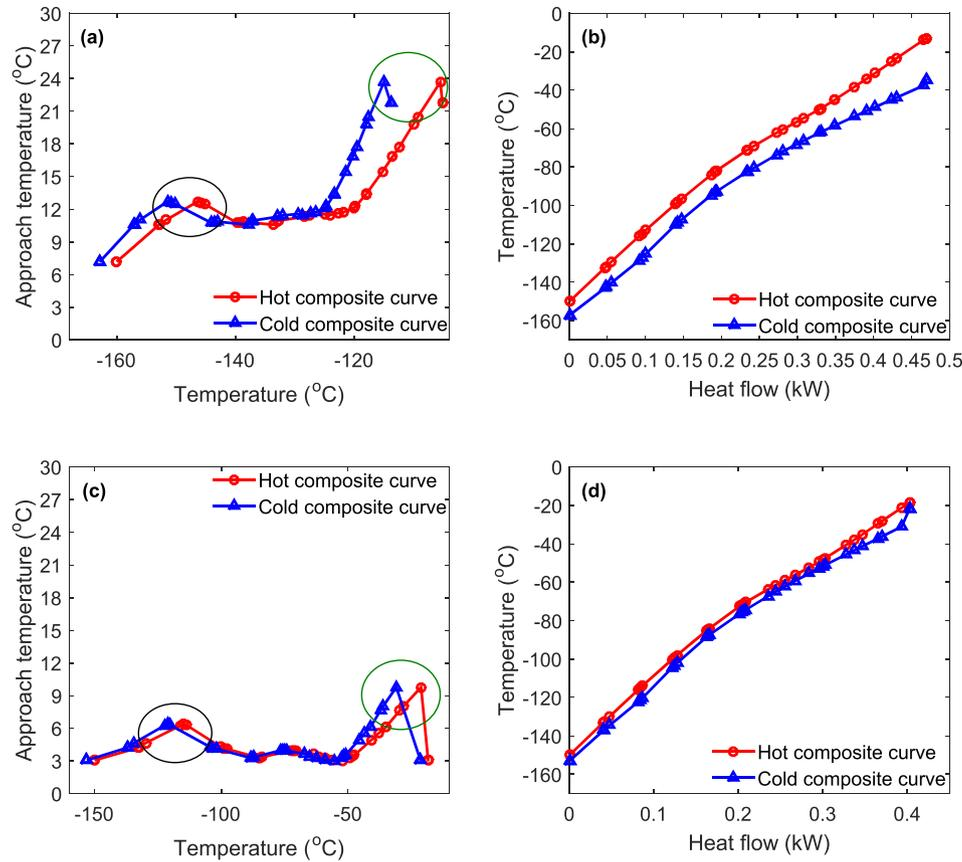
Fig. 6. TDCC and THCC in the main LNG exchanger (CHX-02) of the HFO-MR LNG process, without optimization (a and b) and with optimization (c and d), respectively.
