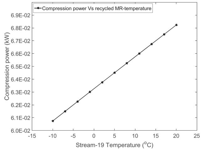
Fig. 4. Relationship between required compression energy and inlet MR temperature.
