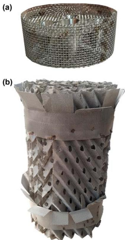
Fig. 6. (a) Liquid distributor and (b) Hanbal's structured packing.
