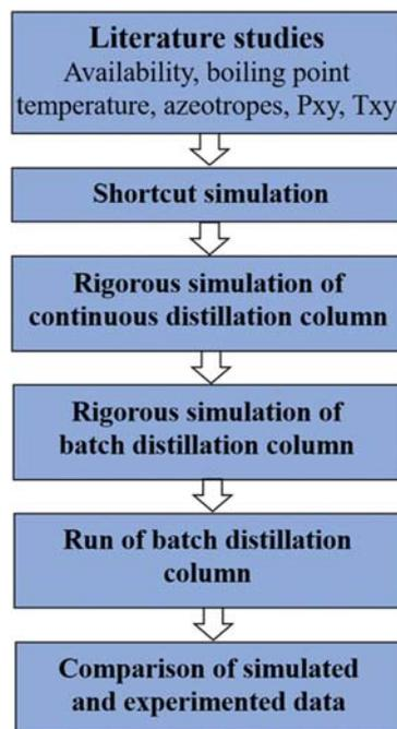
Fig. 1. Systematic procedure of batch distillation design.
