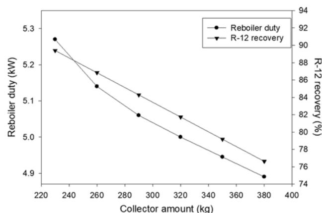
Fig. 9. Effect of collector amount on reboiler duty and R-12 recovery.
