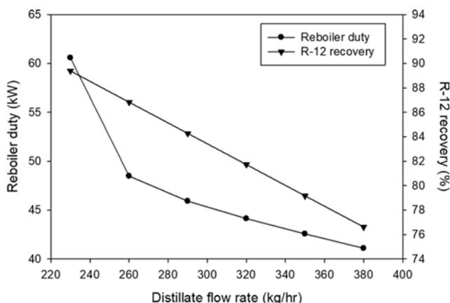
Fig. 5. Effect of distillate flow rate on reboiler duty and R-12 recovery.
