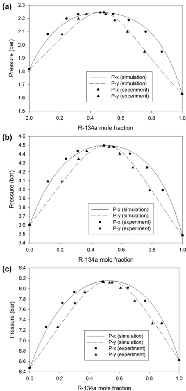
Fig. 2. R-134a+R-12 vapor-liquid equilibrium phase diagrams compared with literature values at (a)  $-15^{\circ}\text{C}$ ; (b)  $5^{\circ}\text{C}$ ; and (c)  $25^{\circ}\text{C}$ .
