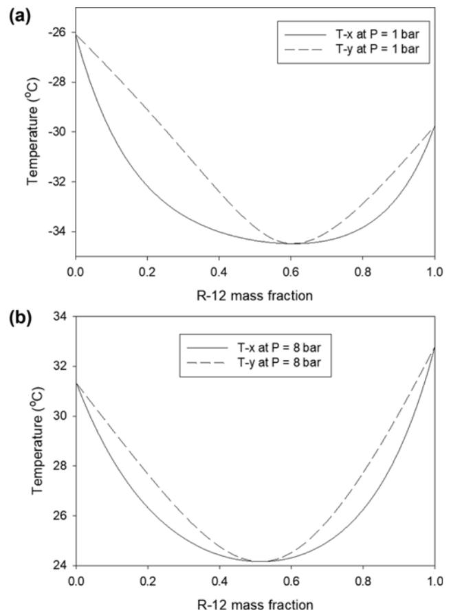
Fig. 3. Temperature vs. composition plot at (a) 1 bar and (b) 8 bar.
