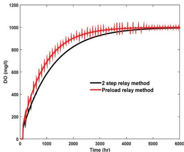
Fig. 10. Closed loop servo response of the ANAMMOX process estimated as FOPTD system for a set point of 1,000 mgO<sub>2</sub>/L.
