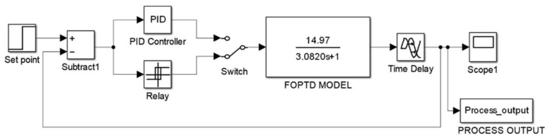
Fig. 6. Closed loop control system for the FOPTD model.
