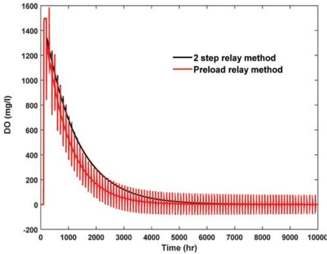
Fig. 11. Closed loop regulatory response of the ANAMMOX process estimated as FOPTD system for a unit step change in the disturbance.
