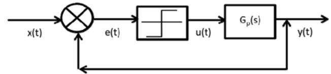
Fig. 1. Block diagram representation of a control system with a relay as the feedback controller for a positive gain system.
