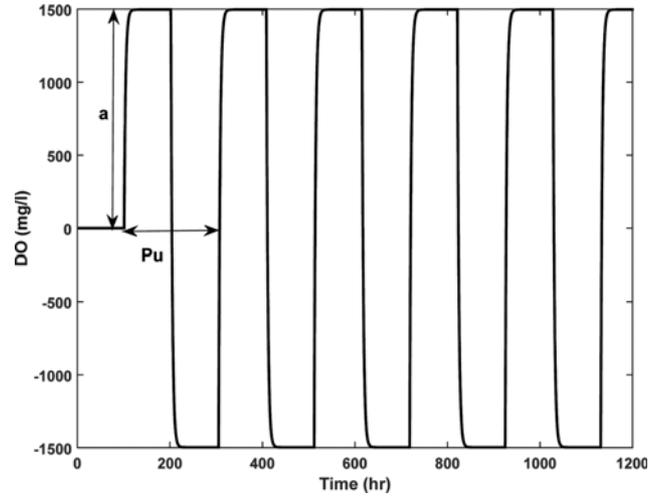
Fig. 7. Limit cycles obtained for the FOPTD model in the absence of noise using the two-step relay.
