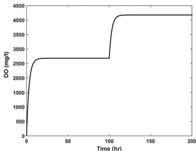
Fig. 3. Process reaction curve corresponding to a change in mass transfer coefficient from  $100$  to  $200 \text{ day}^{-1}$  at  $t=100$  hr in the nonlinear system.
