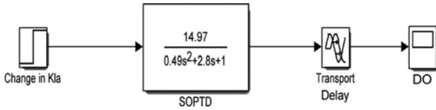
Fig. 5. Open loop control system for the SOPTD model.
