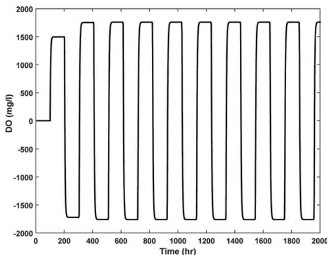
Fig. 8. Limit cycles obtained for the FOPTD model in the absence of noise using the preload relay.
