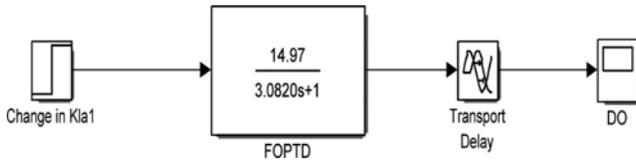
Fig. 4. Open loop control system for the FOPTD model.
