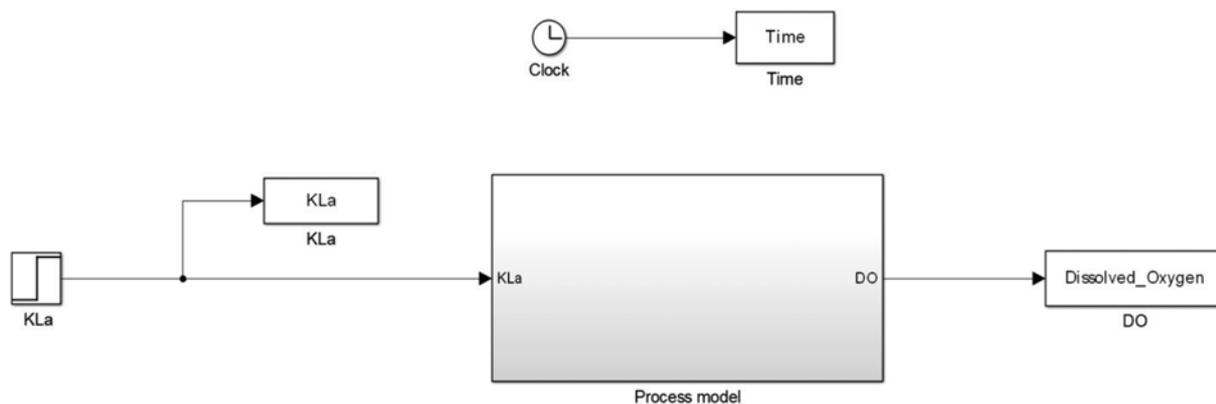
Fig. 2. Open loop control system for the ANAMMOX process.
